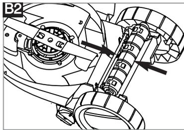
3. Clip the roller together to secure it into position. **(B2)**
